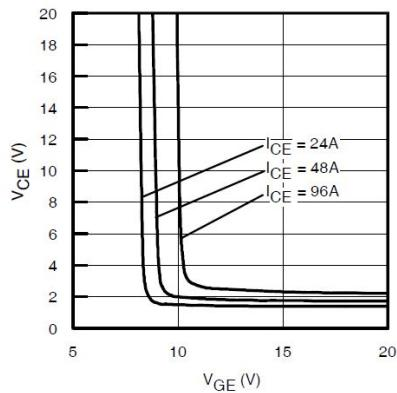
**Fig. 9 - Typical  $V_{CE}$  vs.  $V_{GE}$**
