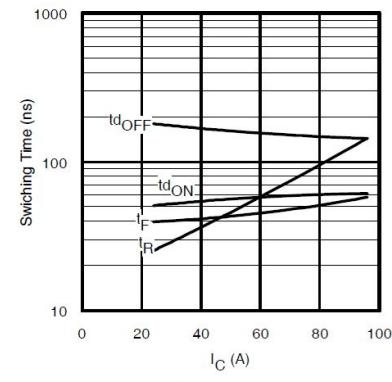
**Fig. 14 - Typ. Switching Time vs.  $I_C$**
