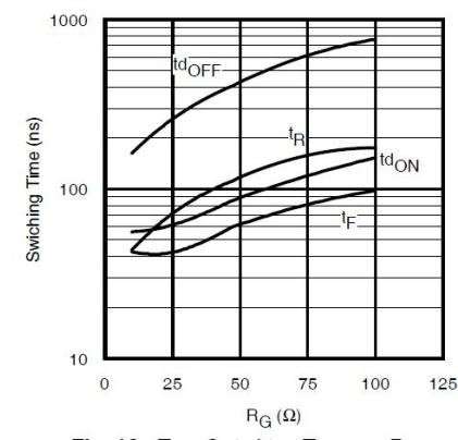
**Fig. 16 - Typ. Switching Time vs.  $R_G$**
