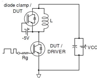
**Fig. 4 - Switching Loss Circuit**
