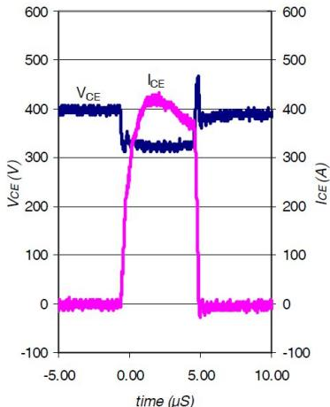
Fig. 10 - Typ. S.C. Waveform
