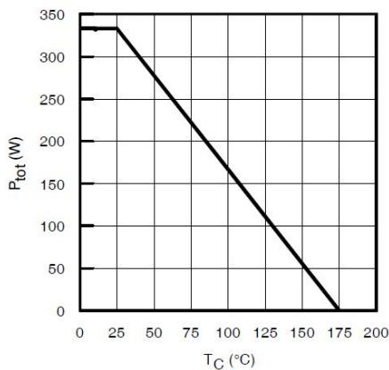
**Fig. 2 - Power Dissipation vs. Case Temperature**
