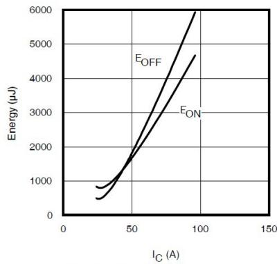
**Fig. 13 - Typ. Energy Loss vs.  $I_C$**
