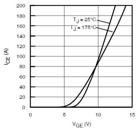
**Fig. 12 - Typ. Transfer Characteristics**
