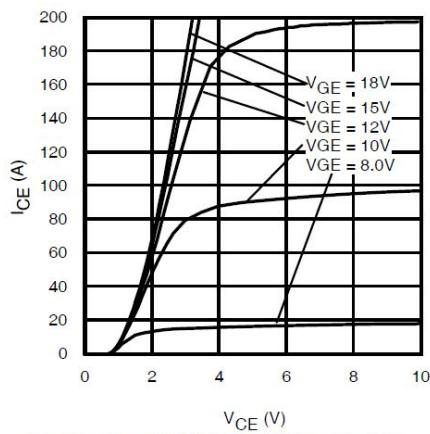
**Fig. 5 - Typ. IGBT Output Characteristics**
