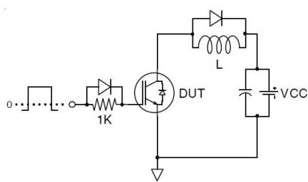
**Fig. 1 - Gate Charge Circuit (turn-off)**
