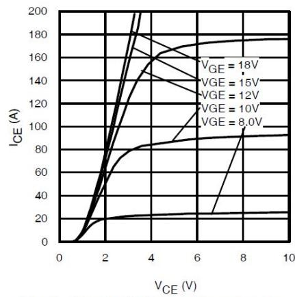
**Fig. 6 - Typ. IGBT Output Characteristics**
