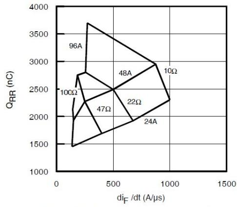
**Fig. 20 - Typ. Diode  $Q_{RR}$  vs.  $dI_F/dt$**
