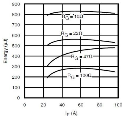
**Fig. 21 - Typ. Diode  $E_{RR}$  vs.  $I_F$**
