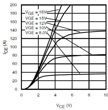
**Fig. 7 - Typ. IGBT Output Characteristics**
