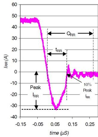
Fig. 9 - Typ. Diode Recovery Waveform
