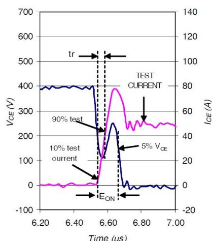
**Fig. 8 - Typ. Turn-on Loss Waveform**
