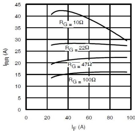
**Fig. 17 - Typ. Diode  $I_{RR}$  vs.  $I_F$**
