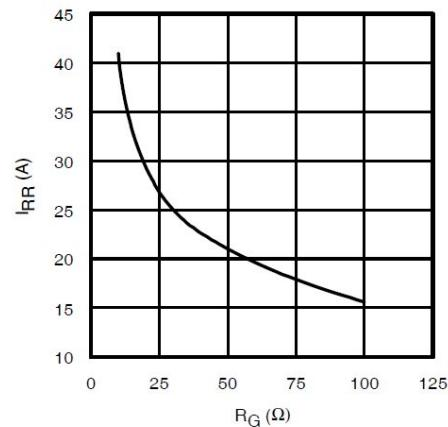
**Fig. 18 - Typ. Diode  $I_{RR}$  vs.  $R_G$**
