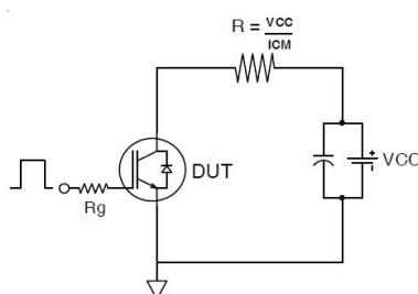
**Fig. 5 - Resistive Load Circuit**
