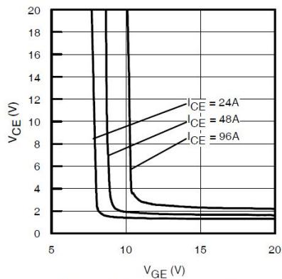
**Fig. 10 - Typical  $V_{CE}$  vs.  $V_{GE}$**
