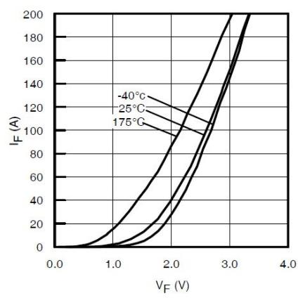
**Fig. 8 - Typ. Diode Forward Characteristics**
