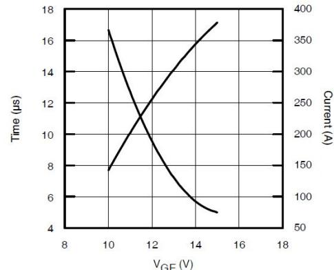
**Fig. 22 -  $V_{GE}$  vs. Short Circuit Time**
