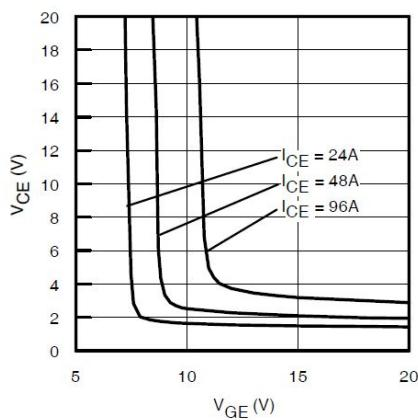
**Fig. 11 - Typical  $V_{CE}$  vs.  $V_{GE}$**
