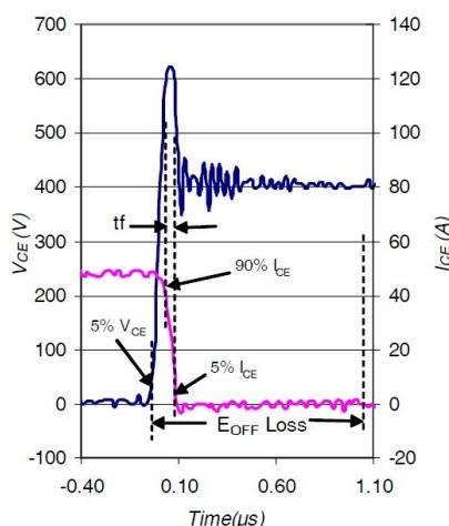
**Fig. 7 - Typ. Turn-off Loss Waveform**
