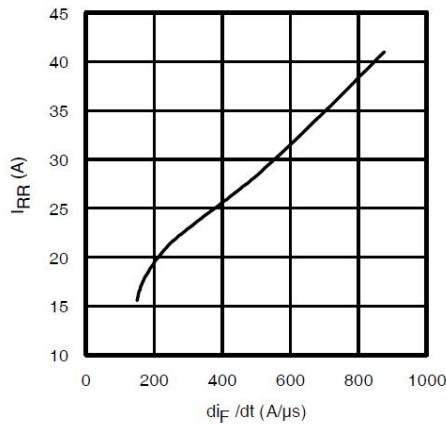
**Fig. 19 - Typ. Diode  $I_{RR}$  vs.  $dI_F/dt$**
